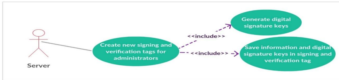
Figure 6 Use Case Diagram for the Creation of New Administrators (Interaction with Server).
