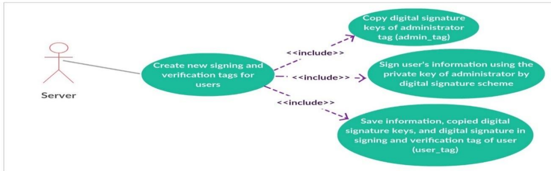
Figure 9 Use Case Diagram for Creating New Users (Interaction with Server).
